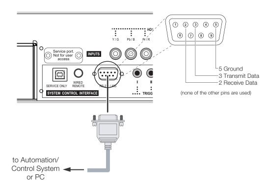
Figure 3-16. RS-232 Control System Connection
